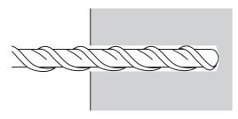
4) Use a device such as a dust pump to clean out concrete dust from the hole.
